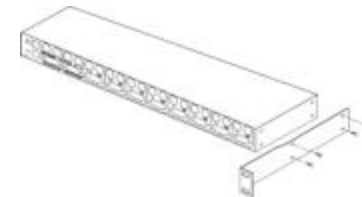
Figure 6: Slave KVM switch and rear bracket attachment
